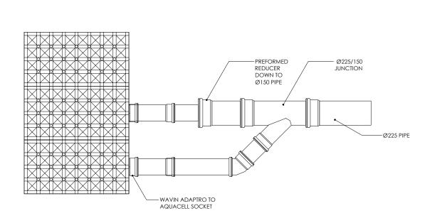
Ø225 TO MULTIPLE Ø150 MANIFOLD CONNECTION TO AQUACELL UNITS
