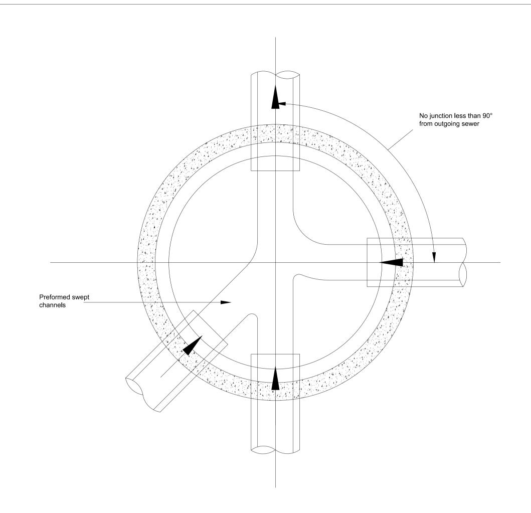
Pipes built into manhole should have a flexible joint as close as feasible to the external face of the structure and the length of the next rocker pipe should be as shown.
