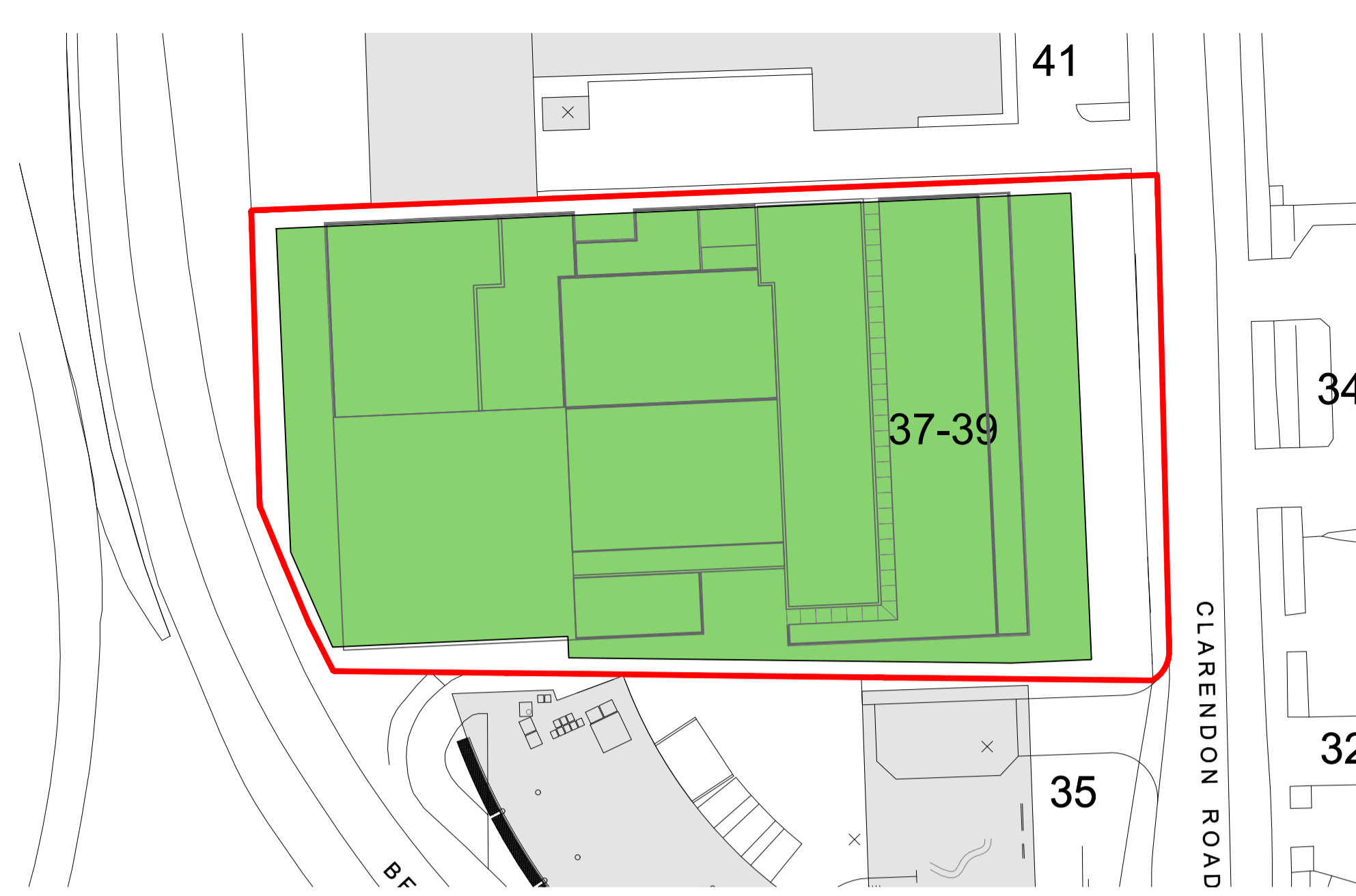
PHASE 3 - PILING AND SUBSTRUCTURE WORKS Once the site is clear, perimeter piling and excavation of the basement structure will be undertaken. The structural frame to the two buildings will be erected in parallel to each other, with the residential building leading the office by 2-3 floors until the office completes.
