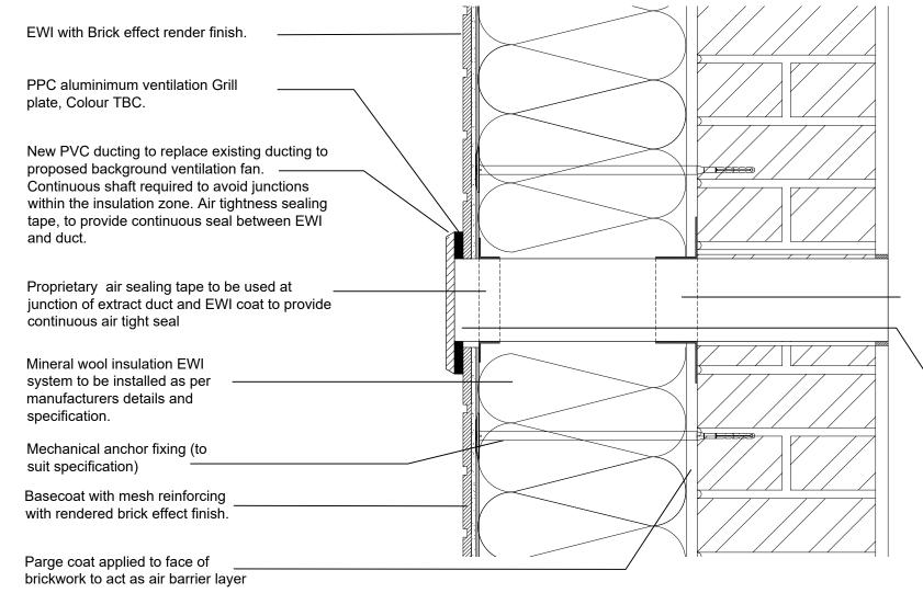
Propriatary air sealing tape or air tightness grommet to be used at junction of extract duct and parge coat. To be lapped under parge coat and sealed to extract duct.
