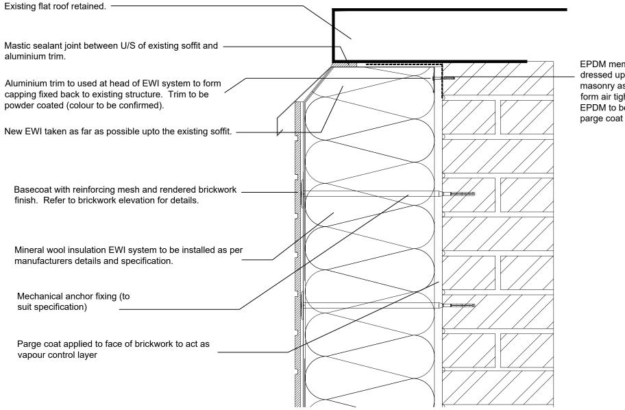
EPDM membrane to be dressed up existing masonry as indicated to form air tightness layer. EPDM to be lapped under parge coat as indicated
