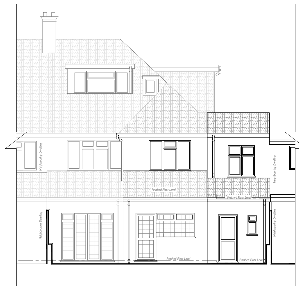
Existing Rear Elevation
