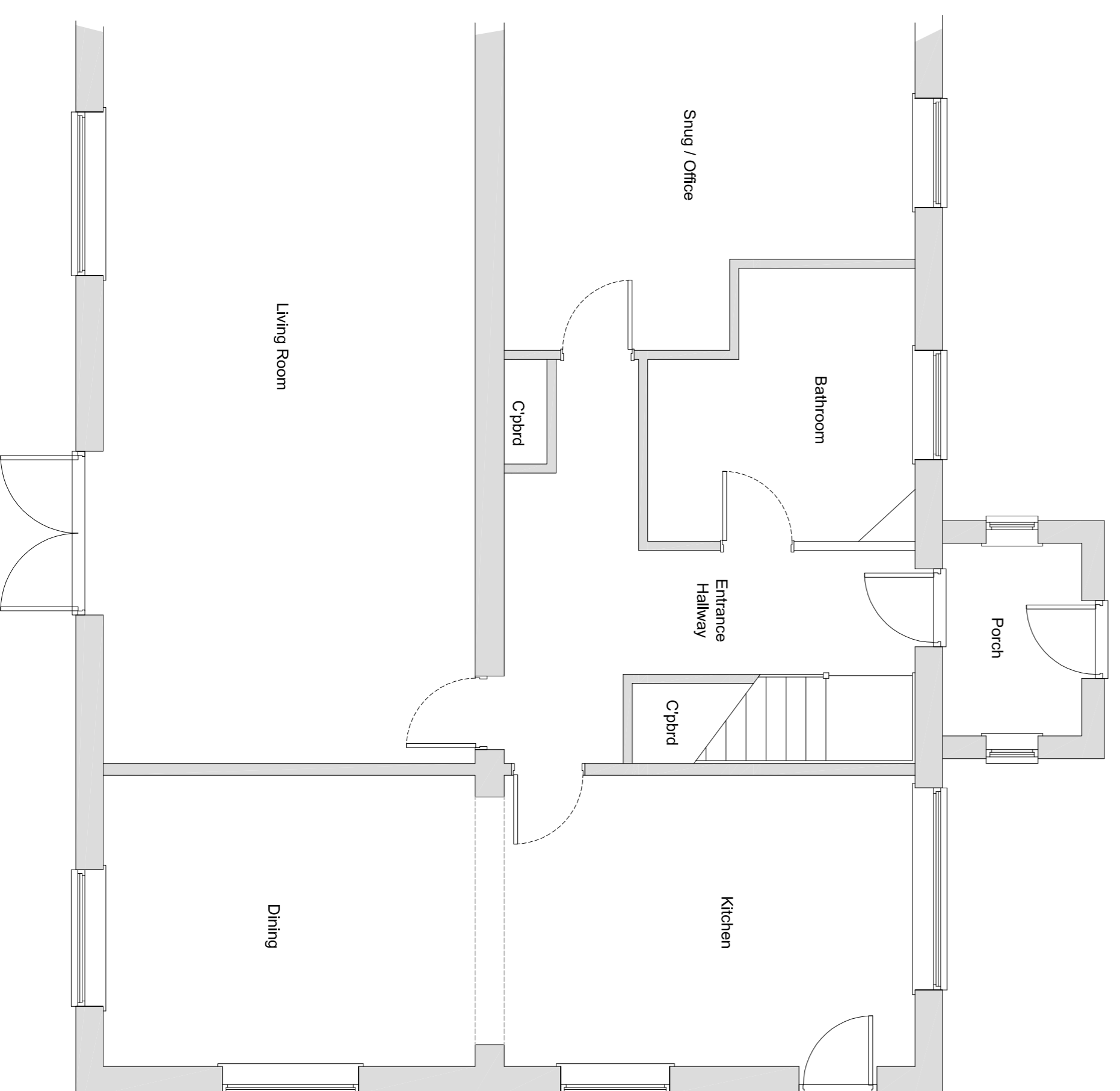
GROUND FLOOR LAYOUT PLAN EXISTING - SCALE 1:50
