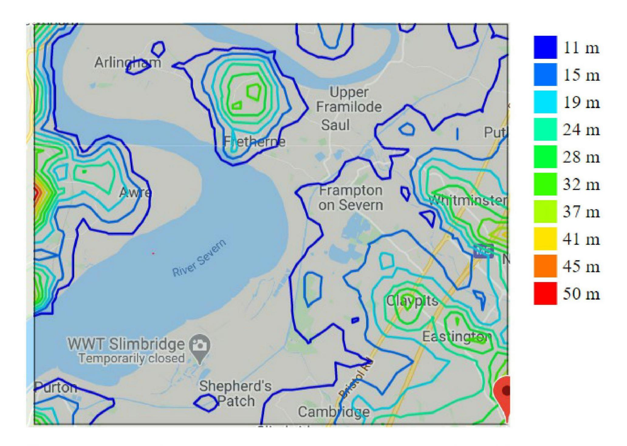
The mapping shows Frampton at 11m AOD. But the higher land at 28mAOD straddles the Arlingham loop forming a natural barrier to the progression of any flooding.
