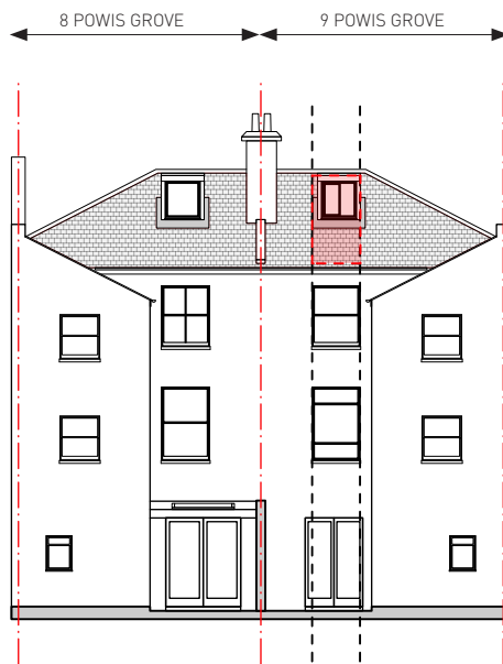
Fig. 06. Existing Elevation Illustrating the Retained Window Pattern.
