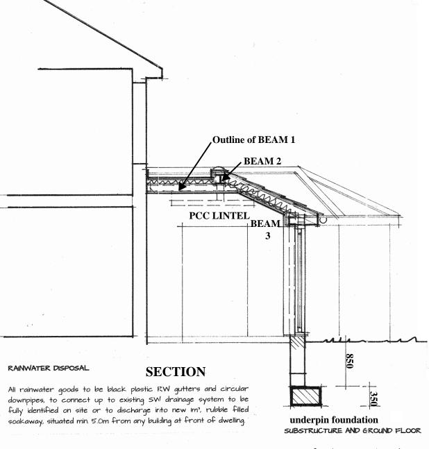
Existing foundations have been determined to be 850mm deep with limited 'toe' projection. Subject to the building inspector agreement, the foundations below the side wall and splay are to be underpinned to extend the depth to 1.2m and to be 450mm in width, extending from the back edge of existing foundation.
