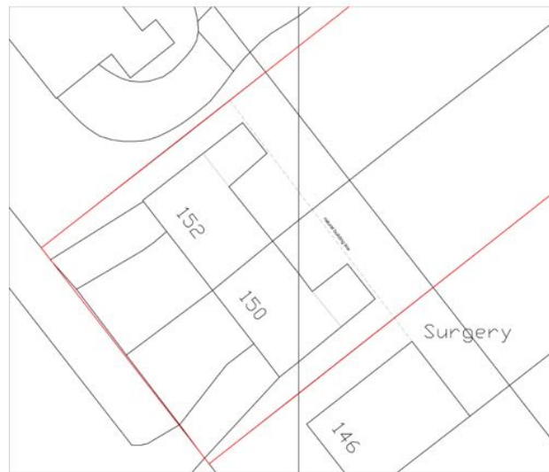
Site Plan showing natural building line
