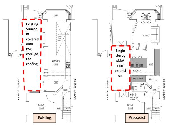
The existing lean-to corrugated pitched roof have a maximum height of 3m, and the proposed extension will have a lean-to pitched roof to a height of maximum of 3.7m fully glazed. The rear extension only is 5.21m long and extends 1.2m from the neighbouring property.
