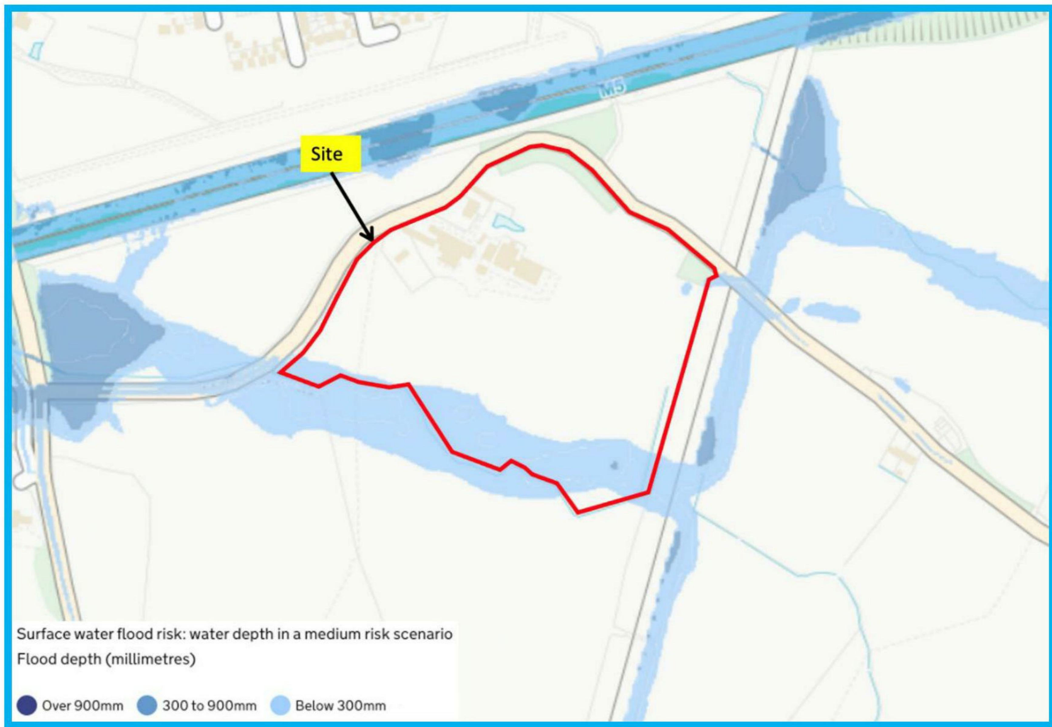
Fig 8 EA Surface Water Flooding Map.
