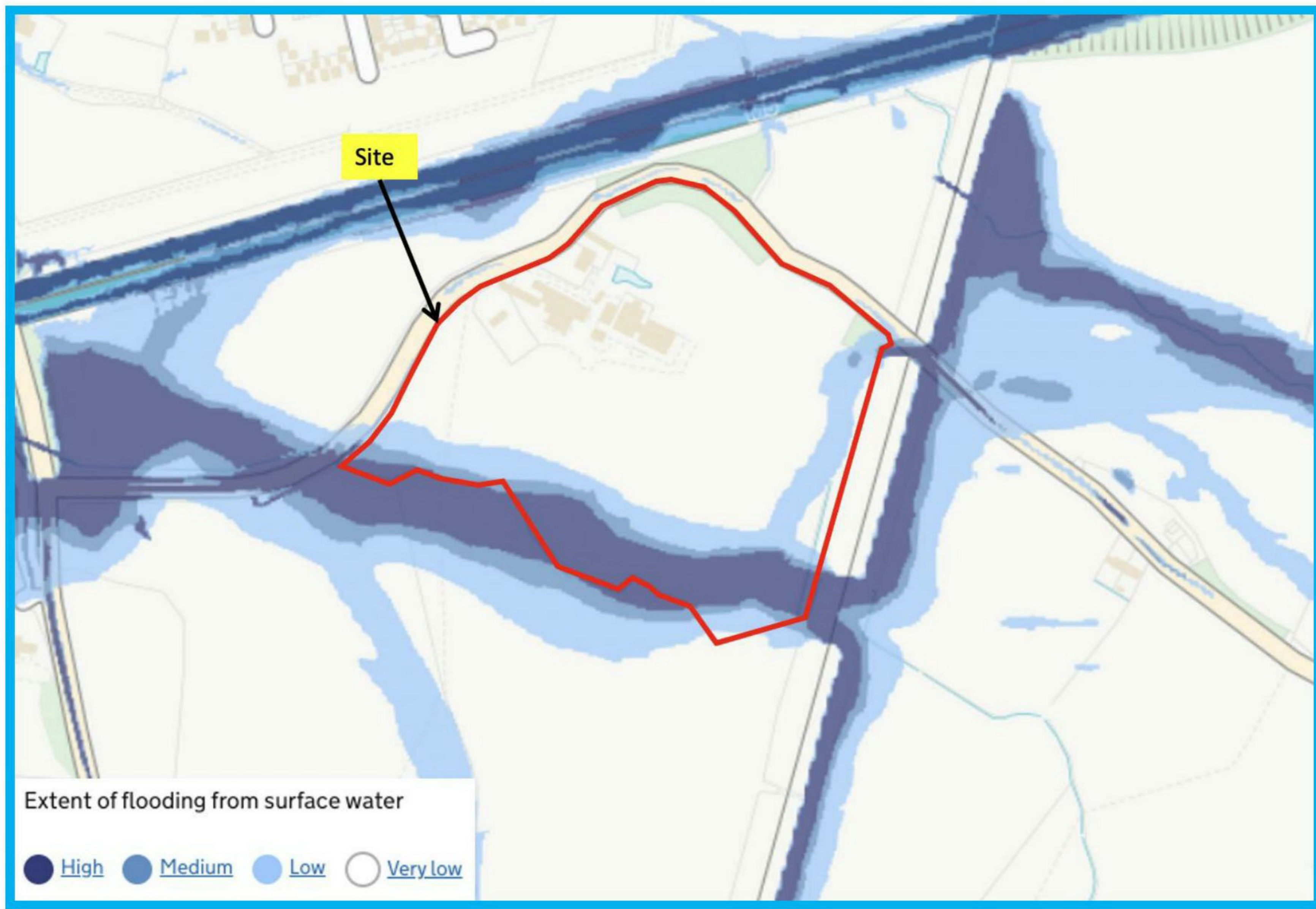
Fig 8 EA Surface Water Flooding Map.
