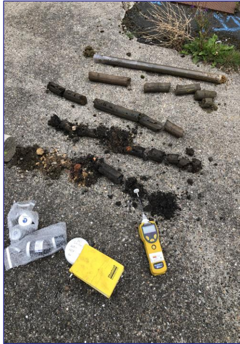
Photographic Plate 11 – WS4 arisings. PID being used to screen arisings during logging.
