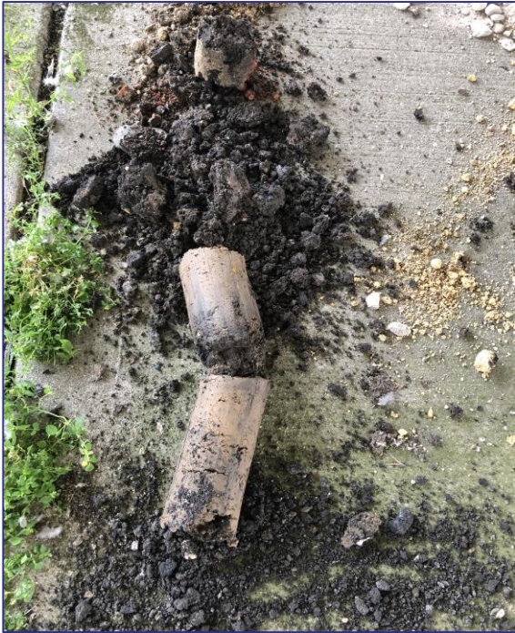
Photographic Plate 7 – WS5 arisings, Made Ground over Clay.
