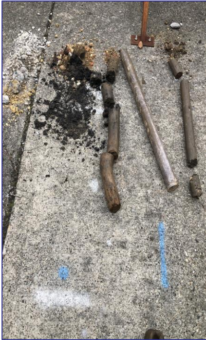
Photographic Plate 5 – WS1 arisings, Made Ground overlying Clay.
