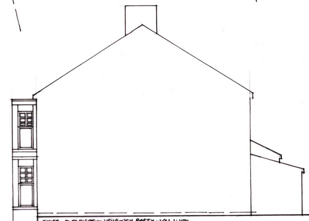
EXISTING ELEVATION THROUGH PARTY WALL 1:100
