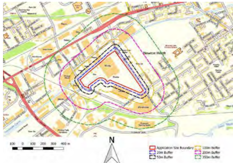
AQM Demolition and construction distance band criteria from the application site boundary
