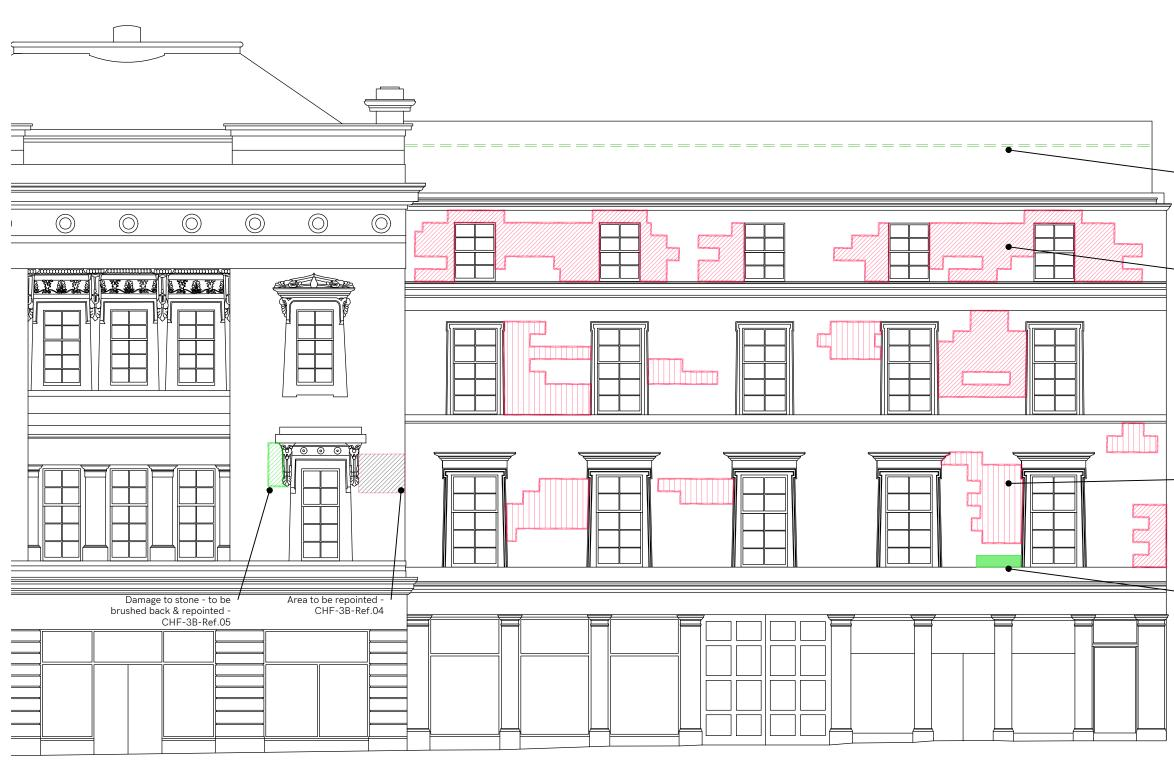
Stone with poor pointing (appears to have had linostone applied over face and joints are not defined)
