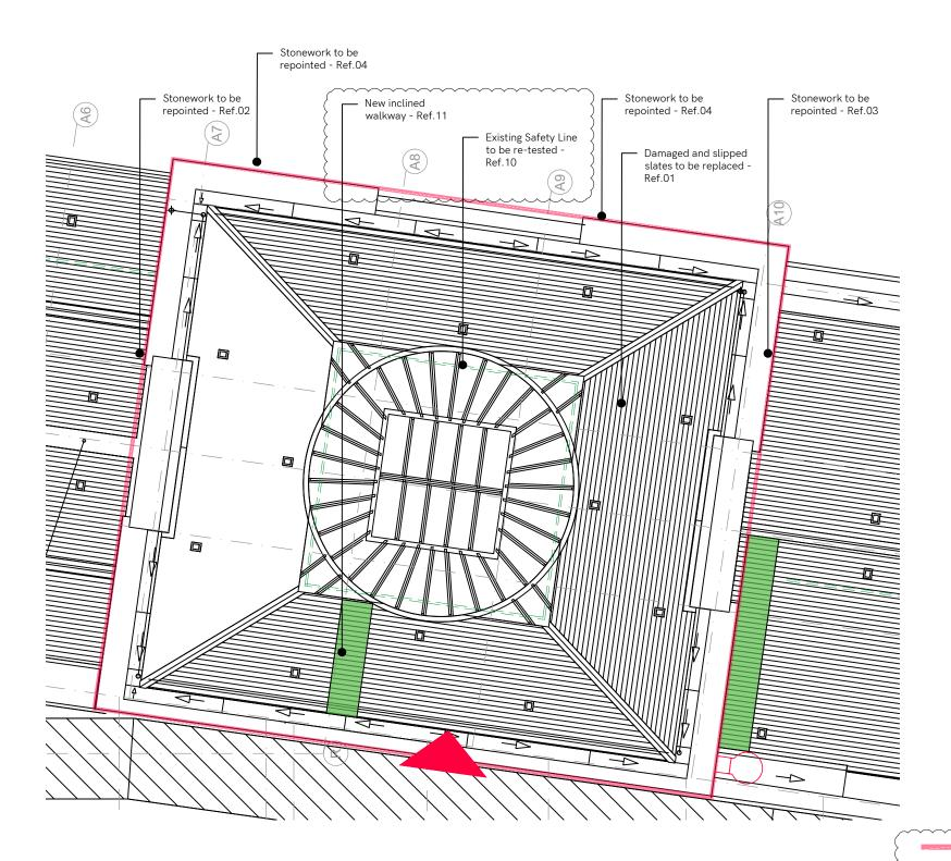
Ref.01 - All slate roofs to be inspected and all slipped and damaged slates to be carefully removed (without damaging adjacent sound slates).
