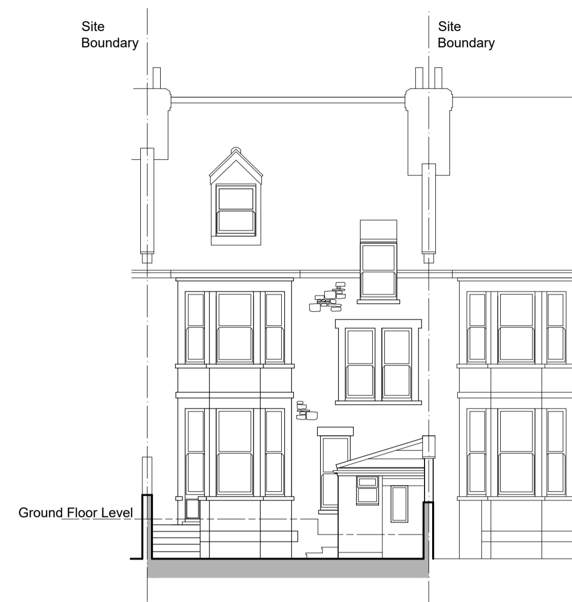
REAR ELEVATION - EXISTING 1:100
