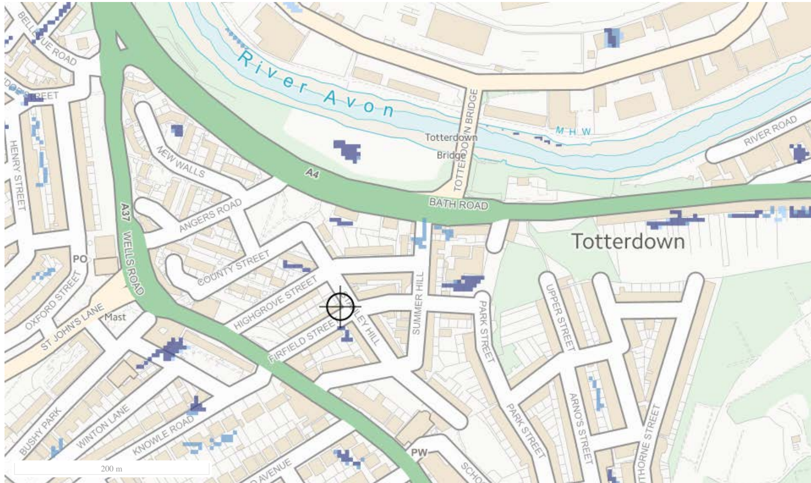
Extent of flooding from surface water
