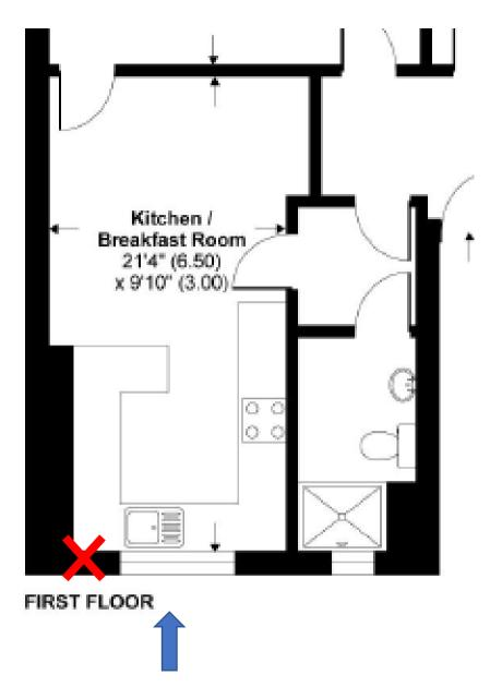
Hole for Flue Extractor to be drilled here, this is the external wall for the property as detailed above. This is the only suitable location for the flue within the kitchen where the gas pipes etc are located.
