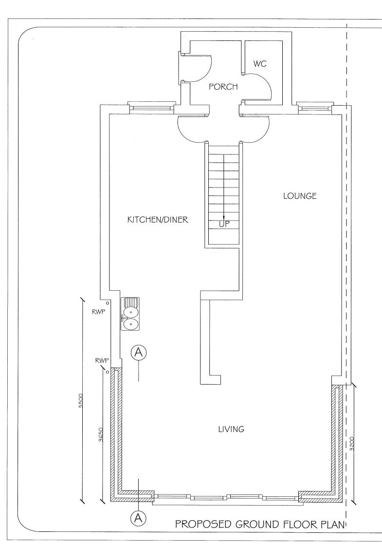
KITCHEN SINK WASTE TO BE 40mm DIAMETER, AND FITTED WITH A 75mm DEEP SEAL TRAP, TAKE TO EXISTING I.C. VIA A BACK INLET GULLEY.
