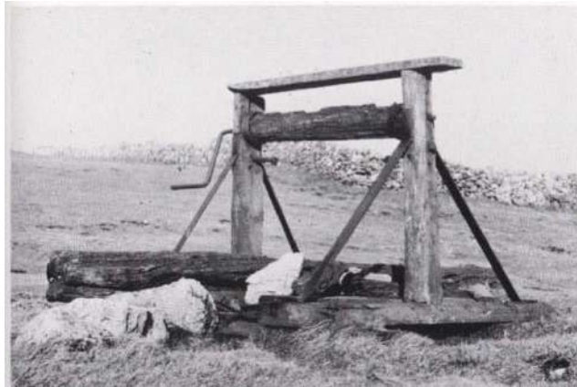
This windlass over a shaft is from a Derbyshire lead mine, but those serving coal pits in Bristol and beyond were almost exactly the same.
