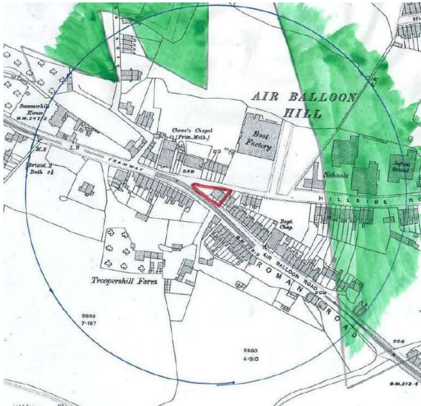
Workings in the Kingswood Great Vein post 1872 according to the Howard Humphreys study (Theme Map H7 (ii)) plotted on the 1918 composite OS county map
