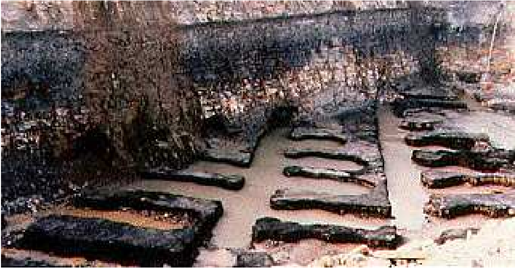
Workings uncovered at Heage in Derbyshire in the 20th century by open cast workings. These were only 20ft (6m) below the surface and show the overburden. Photo courtesy of Robert Bradley.
