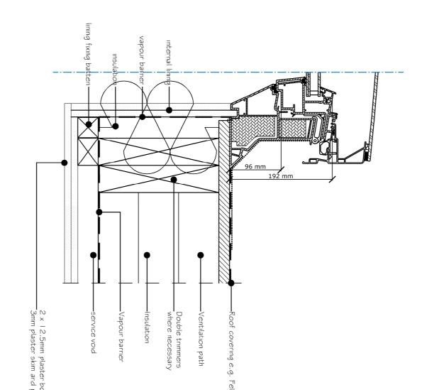
NB. VELUX fixed flat roof window CFP with curved glass cover ISD model number CFP + ISD 1093, U-Value 1.3W/m2K, for roof with a 0 degree pitch, typical size 1000mm x 1000mm
