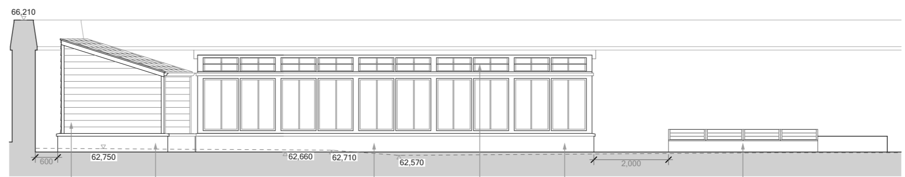
Natural / untreated western red cedar cladding Natural stone plinth to match existing stone wall WEST ELEVATION - 1:100
