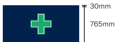
Sign A Cornmarket st fascias Fascia Size: 1,620mm x 765mm + 30mm upstand 3mm aluminium powder coated to match RAL 5013, supplied with fixing rails, 100mm deep. Cross cut from 8mm opal 050 acrylic, pushed through approx 3mm, all acrylic being back lit with LED trays, cross having an applied translucent green vinyl with white keyline.
