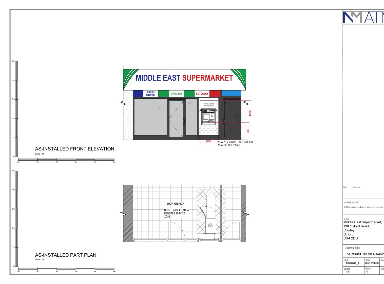
As-Installed Plan and Elevation
