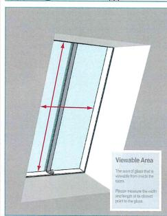
PLEASE NOTE: THE DIFFERENCE BETWEEN AN 'ON THE RAFTER' OR 'BETWEEN THE RAFTER' ROOF WINDOW IS IN THE INSTALLATION, NOT THE ROOFLIGHT SIZE, AND DEPENDS ON THE BUILD-UP OF YOUR ROOF.
