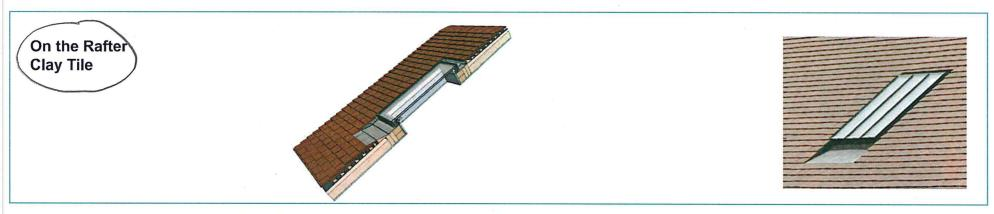
However for some shallow roof build-ups an 'On the Rafter' installation may result in a Rooflight that sits slightly proud if the roofline as illustrated (below left).
