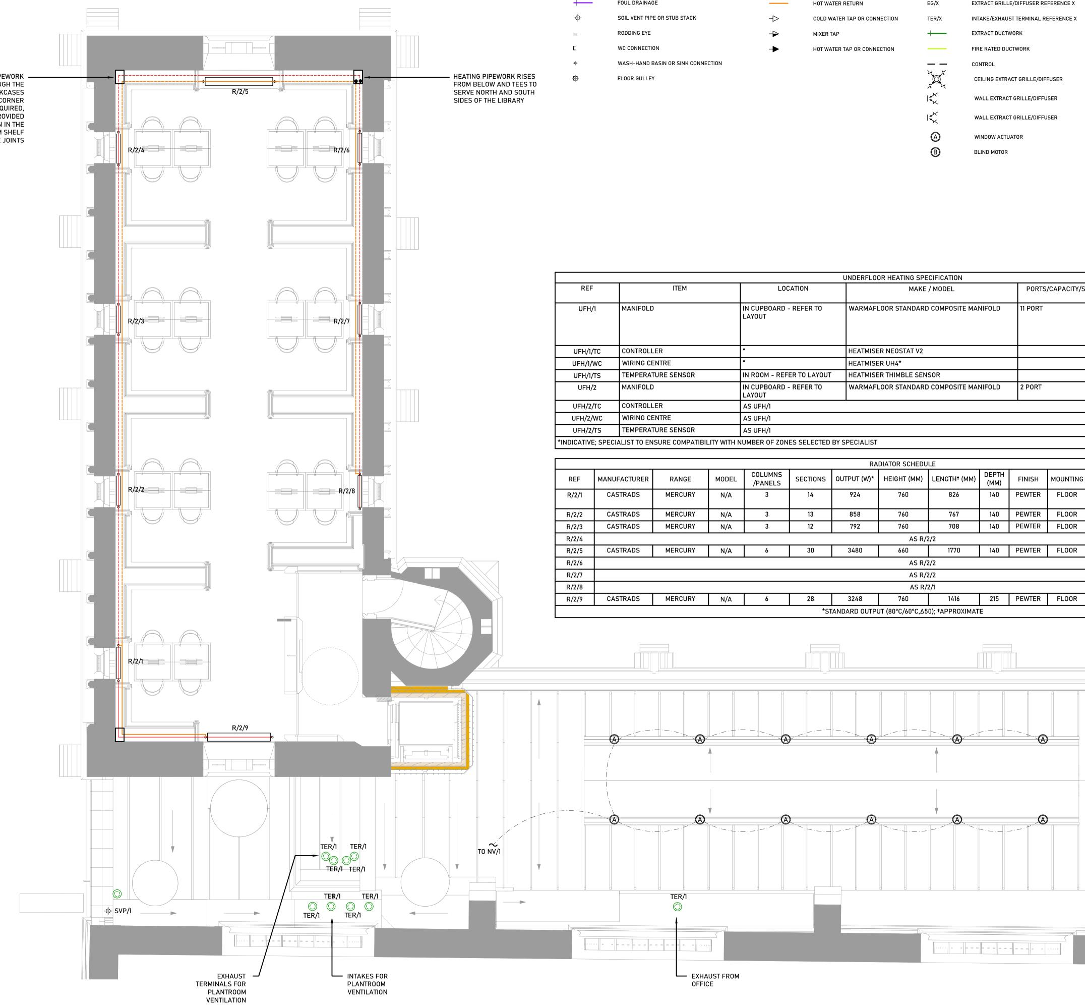
HEATING PIPEWORK PASSES THROUGH THE BASE OF BOOKCASES N.B. WHERE CORNER JOINTS ARE REQUIRED, ACCESS IS TO BE PROVIDED AS SHOWN IN THE BOOKCASE BOTTOM SHELF TO INSPECT THE JOINTS
