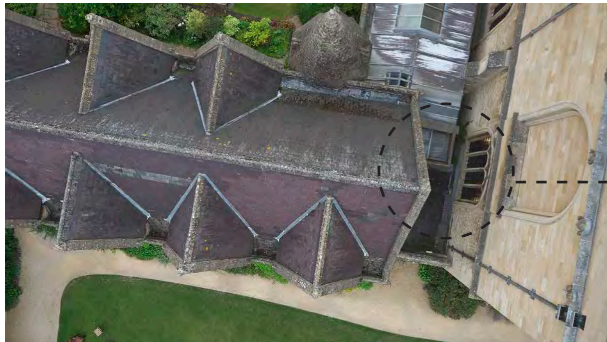
01. Aerial View (north up) to show link-block Bodleian roof interface
