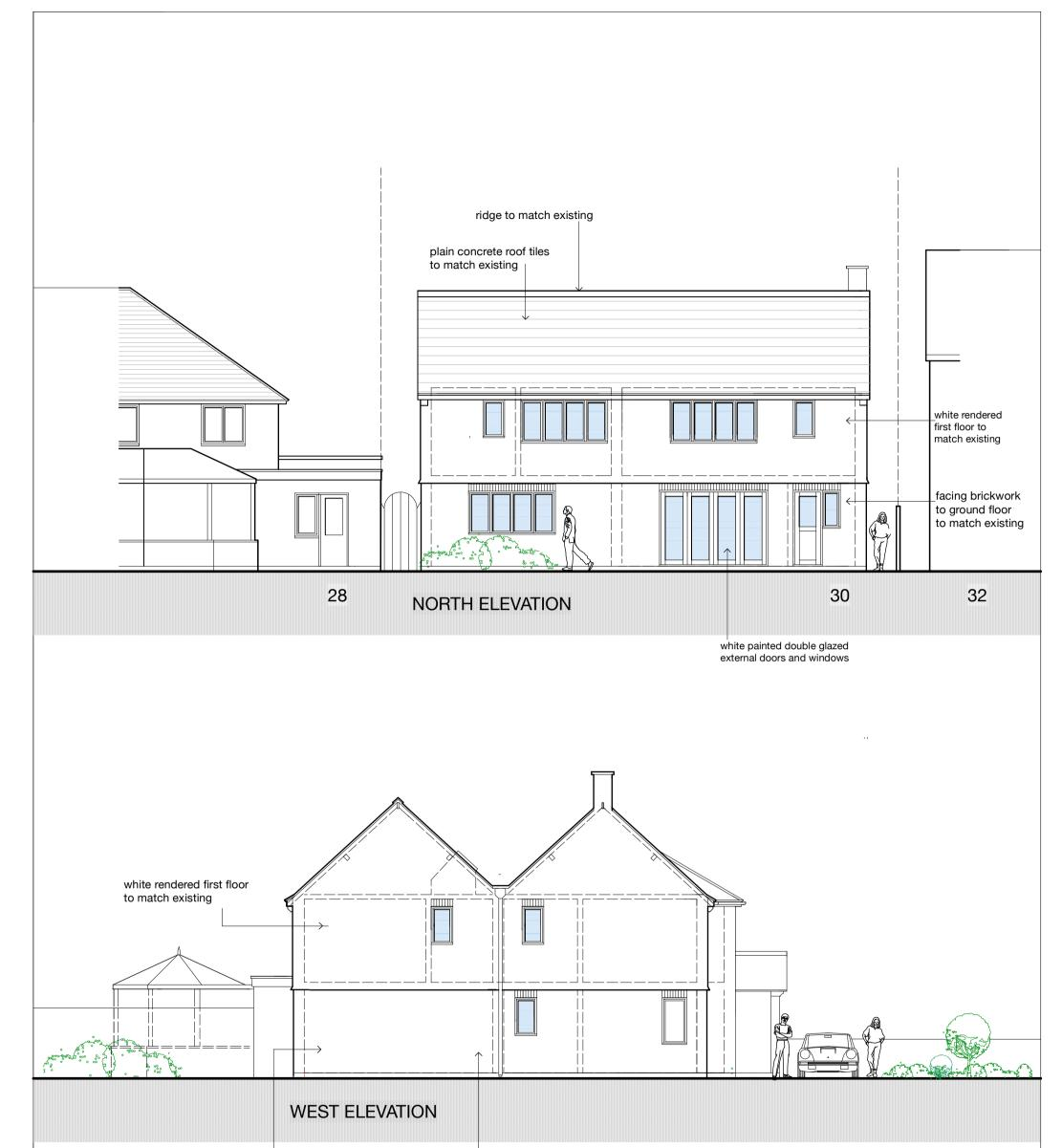
facing brickwork to ground floor to match existing
