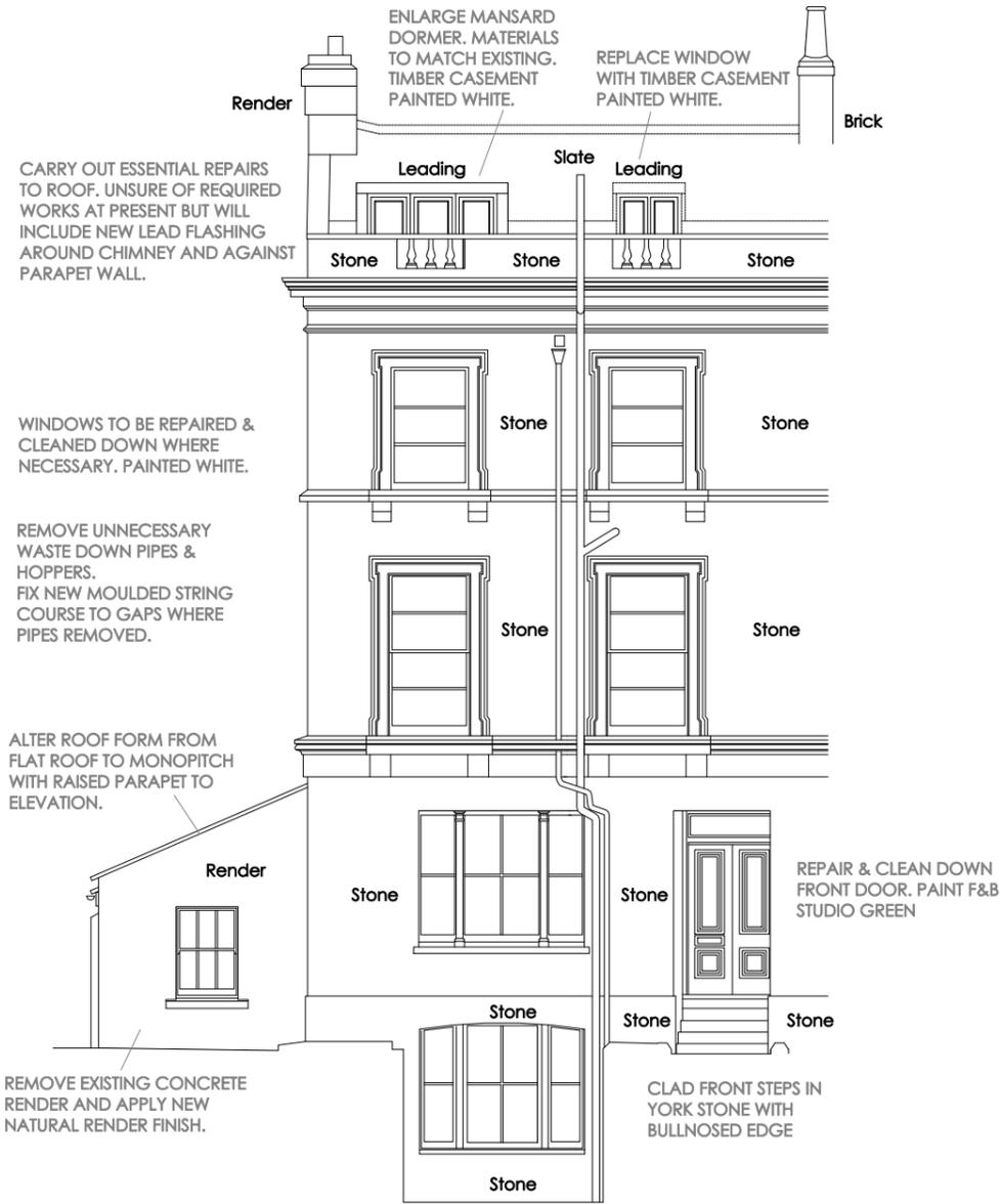
CARRY OUT ESSENTIAL REPAIRS TO ROOF. UNSURE OF REQUIRED WORKS AT PRESENT BUT WILL INCLUDE NEW LEAD FLASHING AROUND CHIMNEY AND AGAINST PARAPET WALL.
