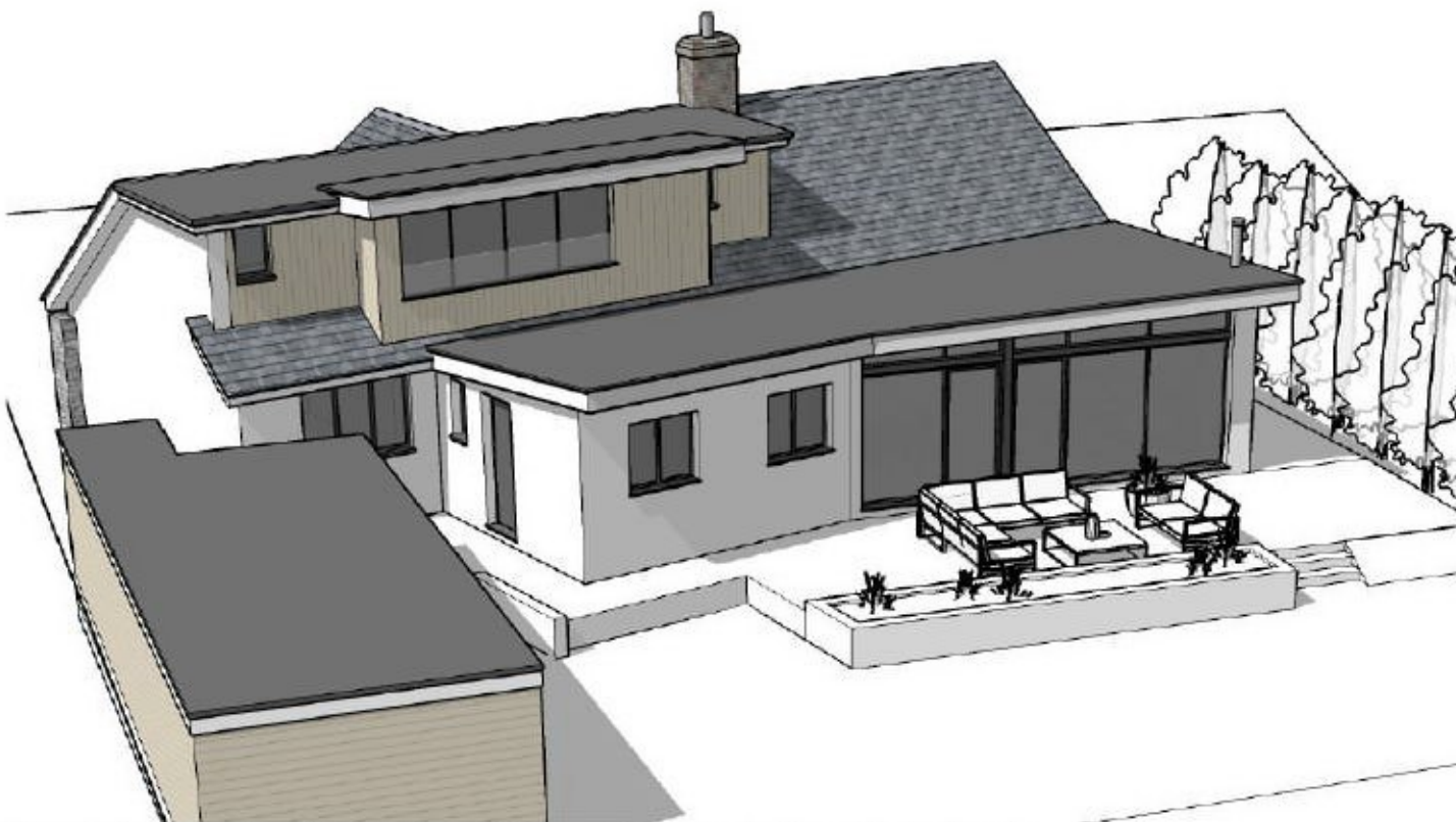
Elevated rear view showing the slightly angled up shallow pitched roofs.
