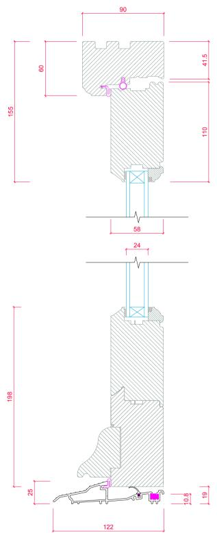
Optimal Door - Open In Feature Mould: Ovolo Vertical Section Standard Aluminium Threshold
