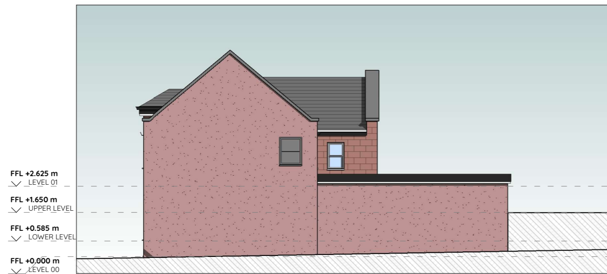
2 NORTH ELEVATION - AS EXISTING 1:100
