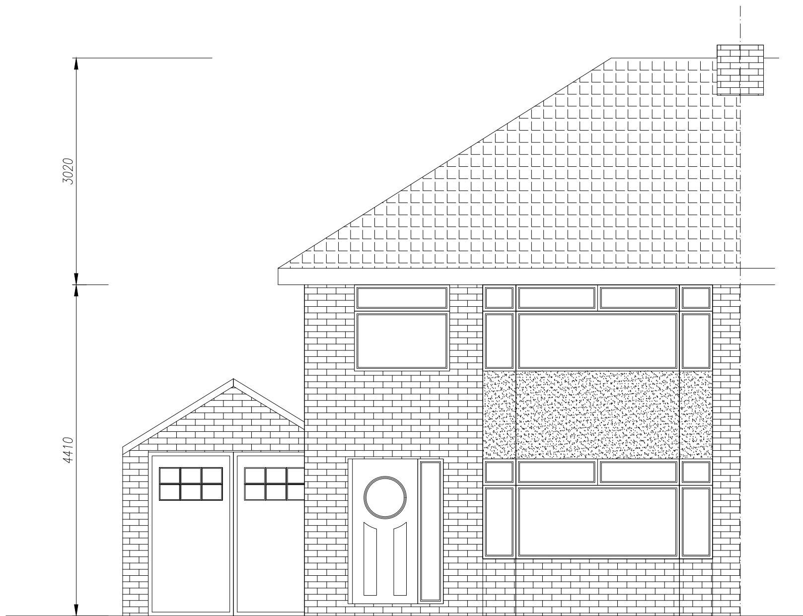
EXISTING FRONT ELEVATION (1:50)
