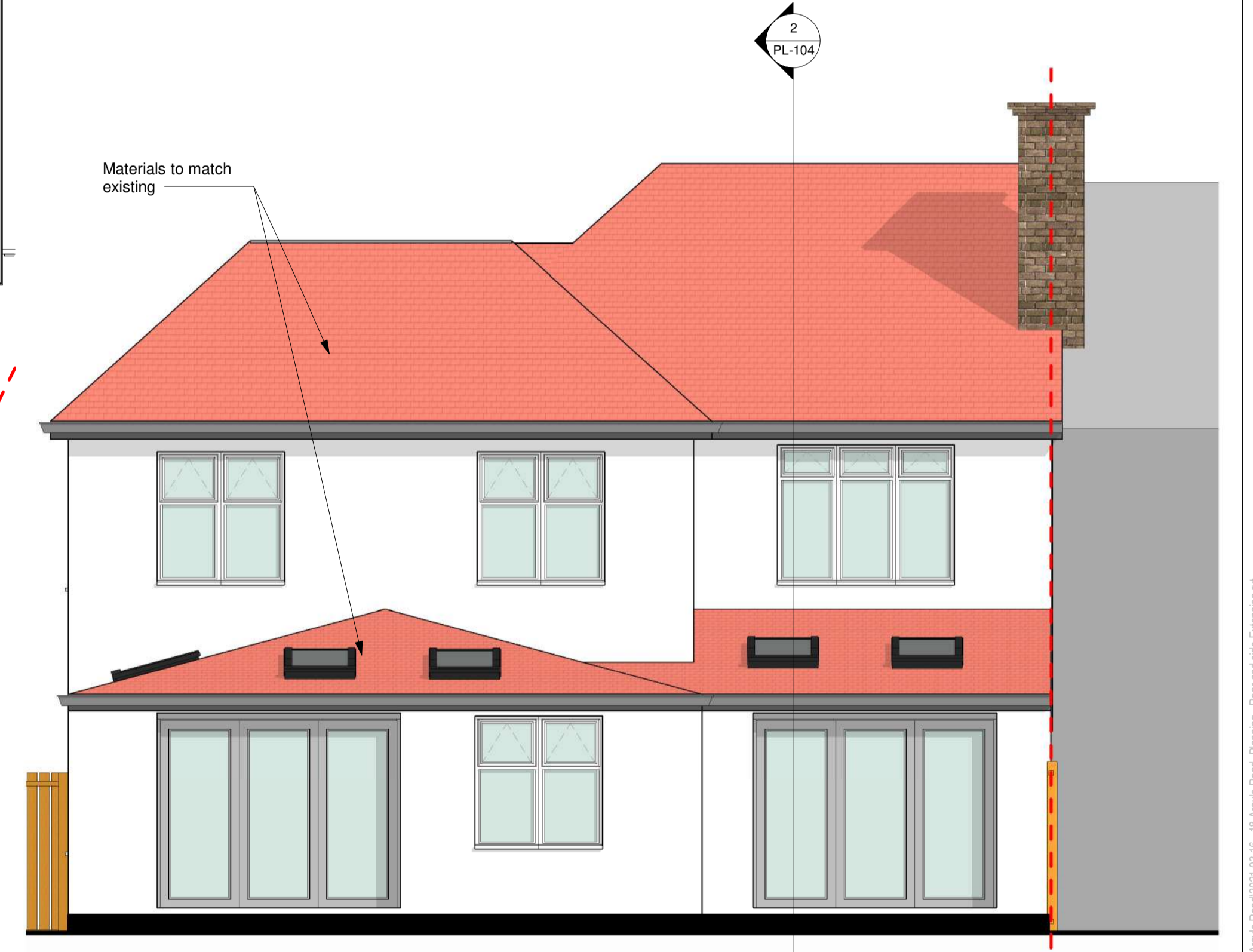
PL - Proposed rear elevation SCALE: 1 : 50 @ A1 1 : 100 @ A3
