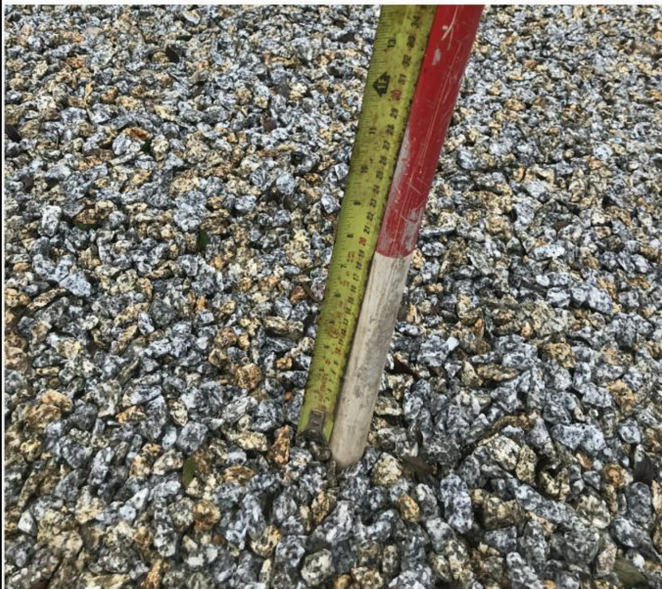
Plate 6 — A view of the rear of the property. The entire rear garden was covered by a gravel cover system of at least 300mm which was considered suitable for breaking the contamination pathway.
