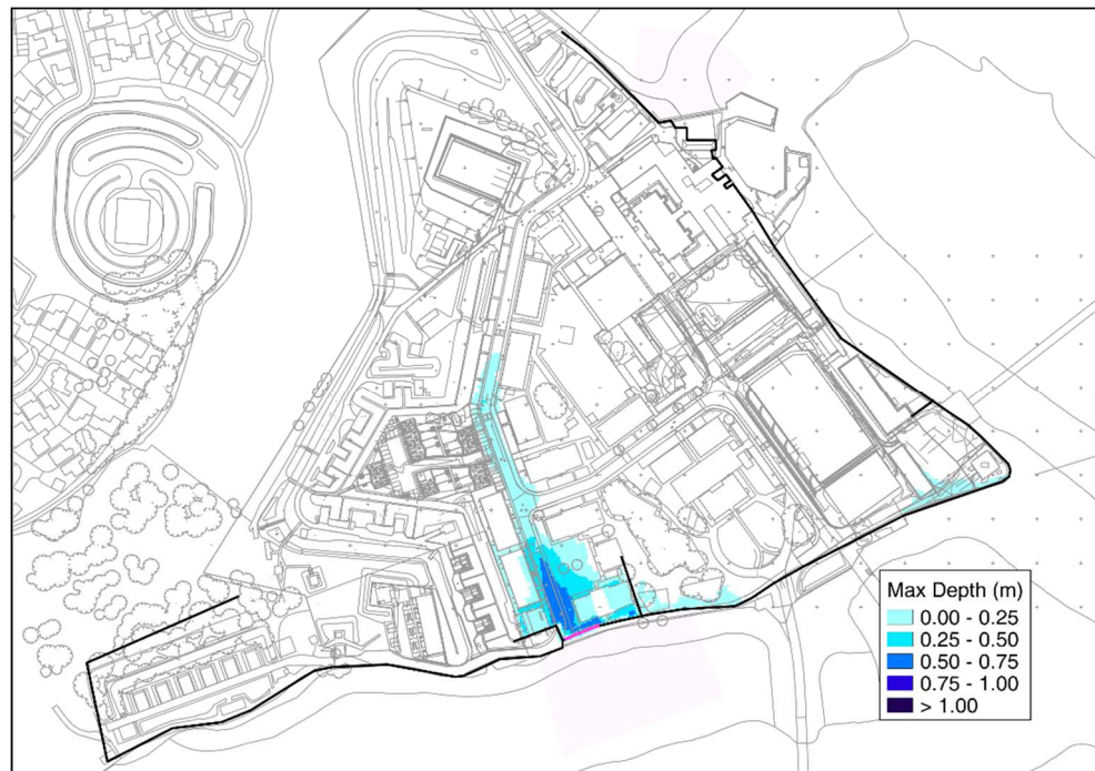
Figure 9 - Maximum depth of flooding resulting from Breach B for the Design Event, including wave overtopping.
