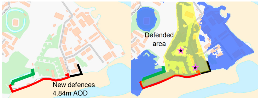
Extended SFR defences at 4.84m AOD Enlarged defended area 2115 AD 0.5% AEP
