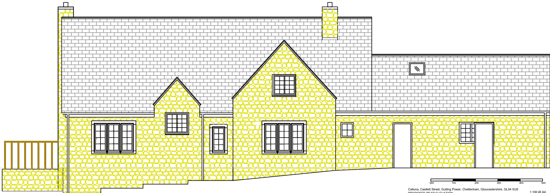
Calluna, Castlett Street, Culling Power, Cheltenham, Gloucestershire, GL54 5US PROPOSED REAR ELEVATION 1:100 @ A4
