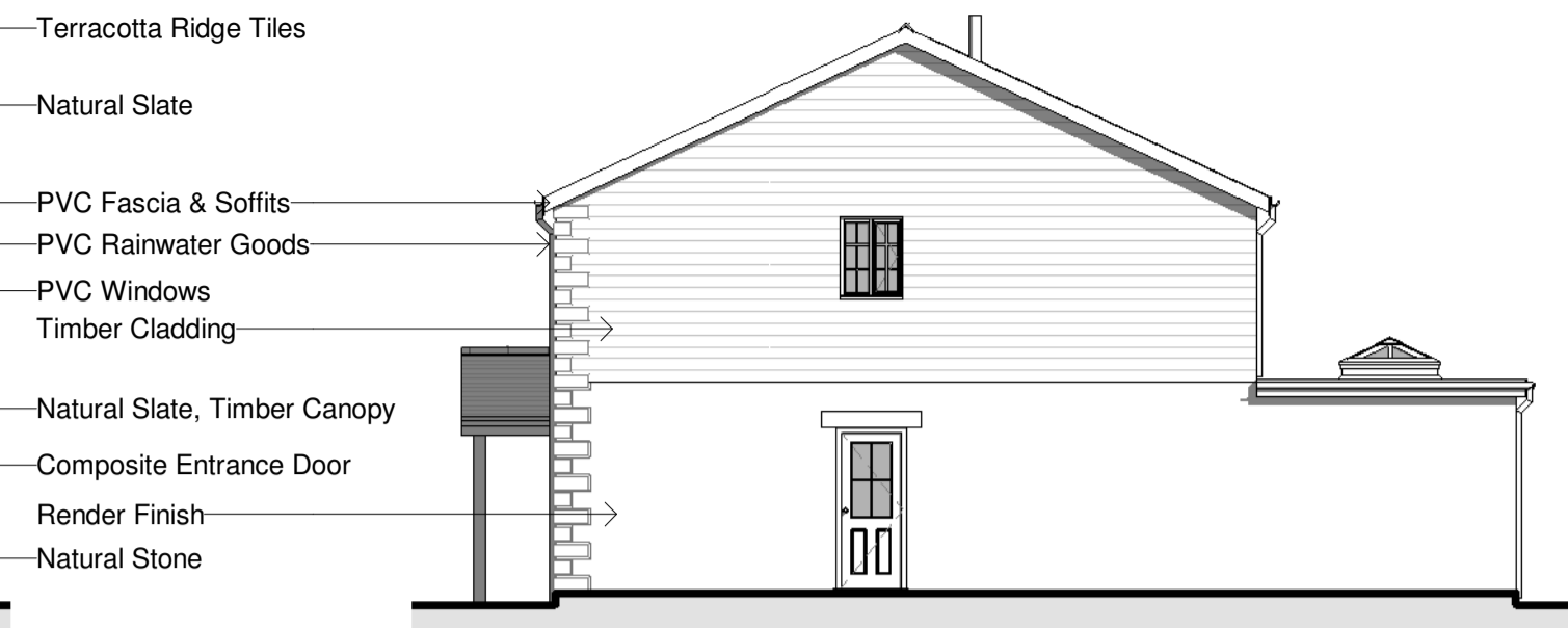
3 North West Elevation 1 : 100
