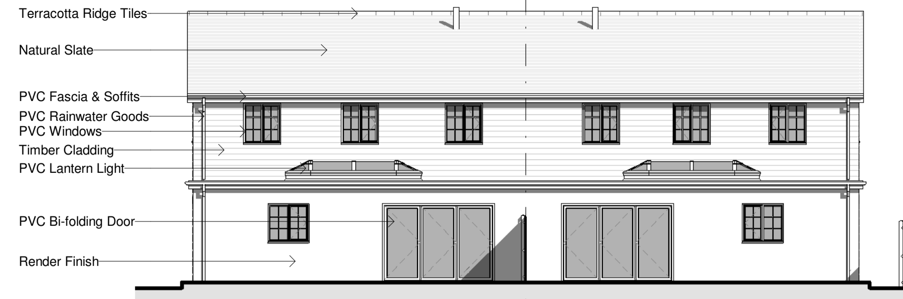
4 South West Elevation 1 : 100
