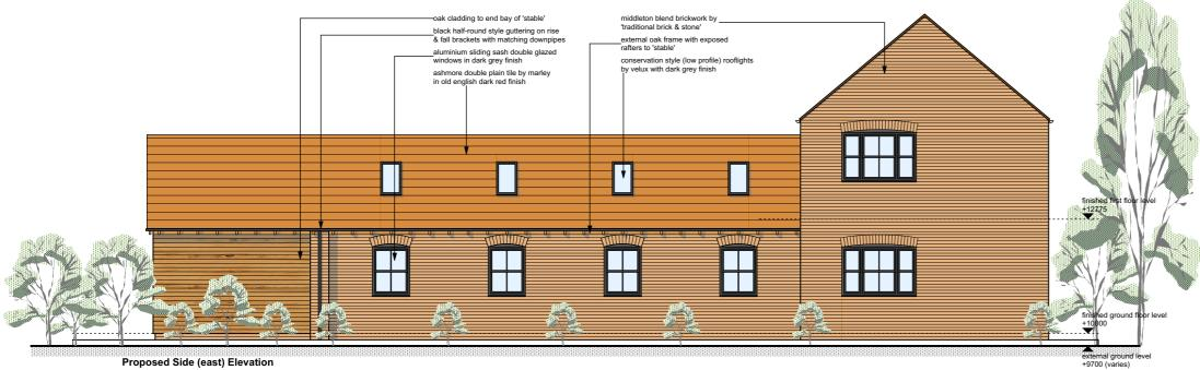
Proposed Side (east) Elevation (scale 1:100)
