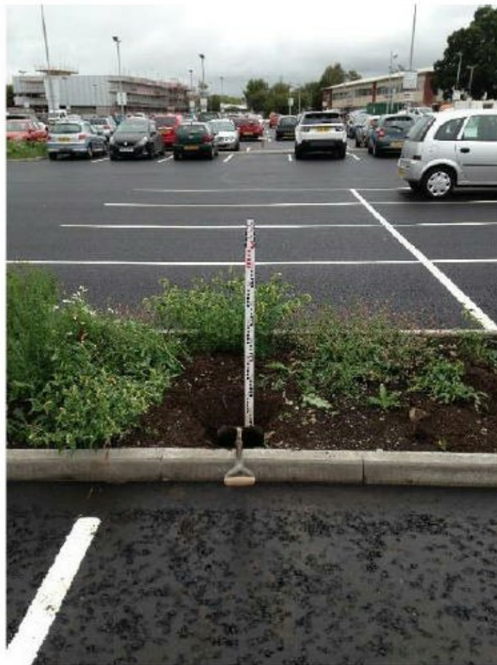
Depth of Cover System at Ground Level and in Relation to Unit / Structure
