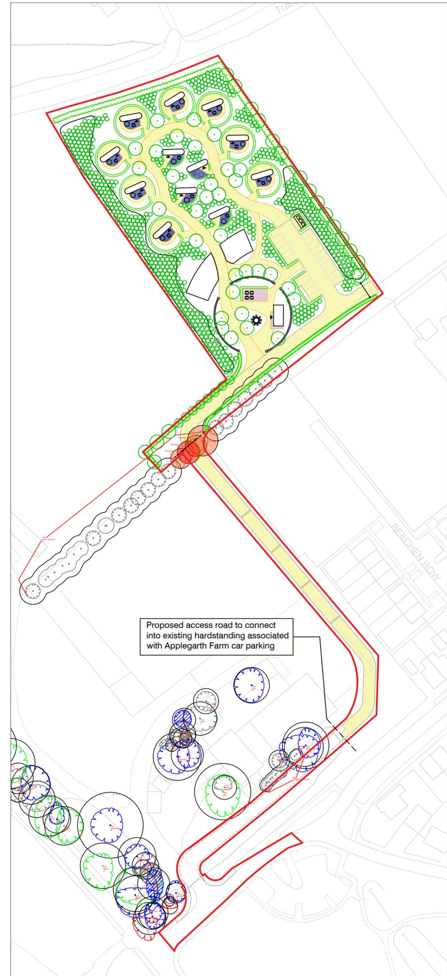
Proposed access road to connect into existing hardstanding associated with Applegarth Farm car parking
