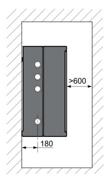
$NOTE: All\ measurements\ are\ millimetres.\ Clearance\ necessary\ for\ the\ installation\ or\ maintenance\ of\ the\ appliance$
