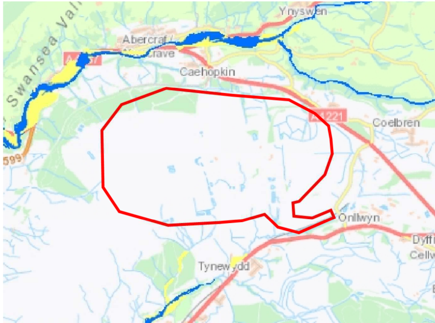
Figure 2: Long term flood risk Development Advice Map for the Nant Helen site. Yellow – Zone B, Blue – Zone C2
