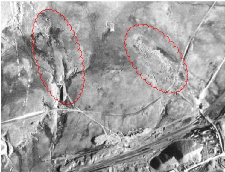
Figure 12 Extract from 1945 aerial photography showing potential 'bell pitting'
