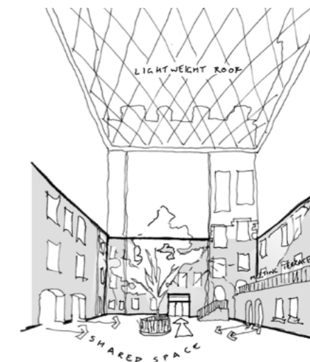
Courtyard roof supported by existing structure
