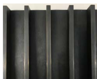
Fabricated diffuser screen
